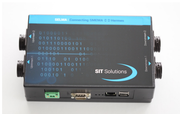
SELMA Connecting SMEMA with IPC Hermes Standard
